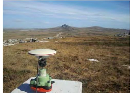
Surveying the new absolute observing pillar using differential GPS at Port Stanley Observatory, Falkland Islands
