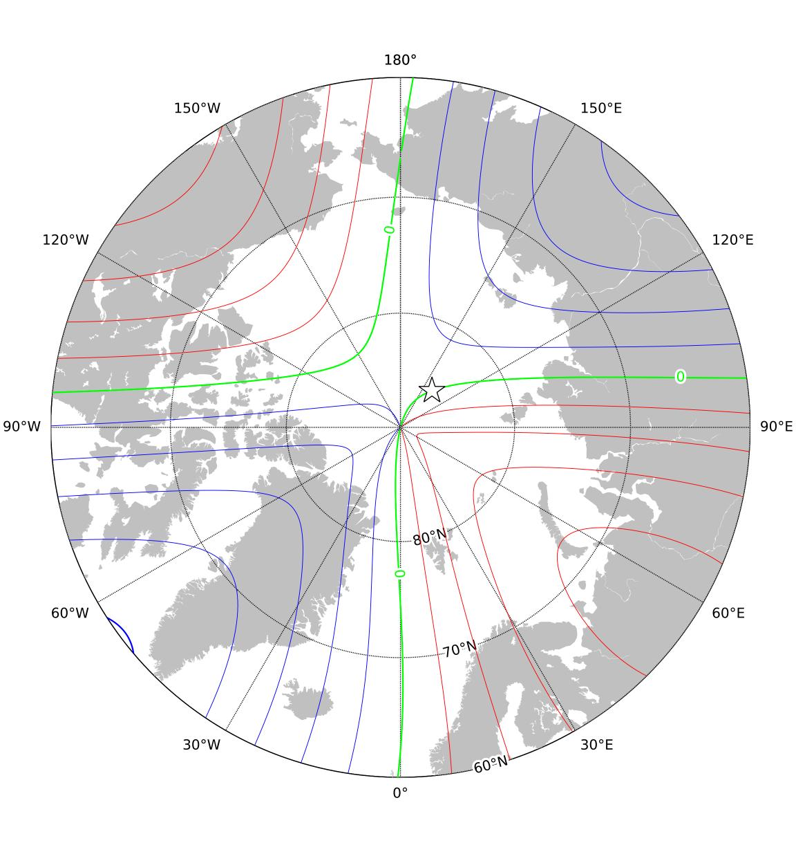
East component (Y) in the region of the north pole at 2025.0 from the World Magnetic Model (WMM) 2025. Red -positive (east), blue - negative (west), green - zero. Contour interval is 1000nT, white star is the location of a magnetic pole and the projection is Polar Stereographic. This is an example of an isodynamic chart. British Geological Survey © UKRI 2024
