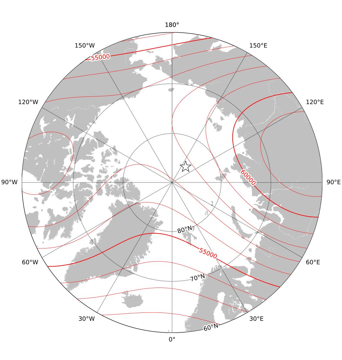
Total Intensity (F) in the region of the north pole at 2025.0 from the World Magnetic Model (WMM) 2025. Contour interval is 1000nT, white star is the location of a magnetic pole and the projection is Polar Stereographic. This is an example of an isodynamic chart.
