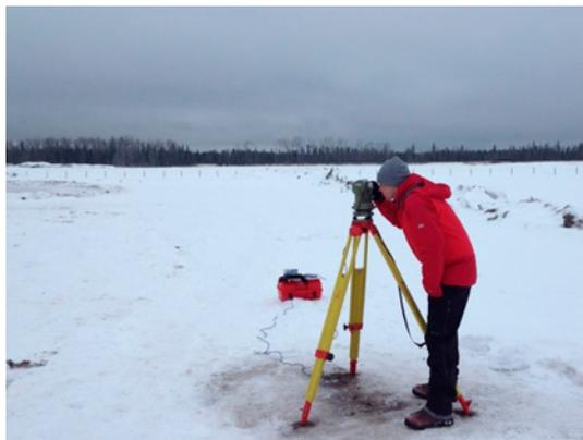
*Magnetic surveying using a D/I theodolite during installation of the Fort McMurray Observatory.*
