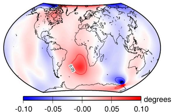
*Declination differences at Earth's surface at 2016.0 between a truncated BGS model and WMM2015.*
