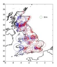
Estimated 1 in 200 year extreme GIC in the transmission system. Spot size is proportional to current into (red) or out of (blue) the ground. Spots are summed GIC at transformer substations
