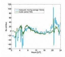
Measured (blue) and modelled (green) geoelectric field at Eskdalemuir for the storm of 2<sup>nd</sup> October 2013. Differences are in part due to local induction effects. Electric field in the north direction is shown
