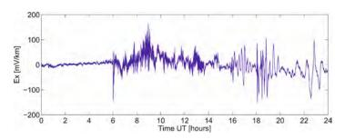
Measured geo-electric field in mV/km at Eskdalemuir observatory, for a magnetically stormy day in 2013 (north component shown)
