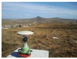
Surveying the new absolute observing pillar using differential GPS at Port Stanley Observatory, Falkland Islands
