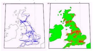
High voltage grid of the UK at 2008 (left) and GIC flowing at major transformers (right) for a hypothetical east-west surface electric field of 1V/km
