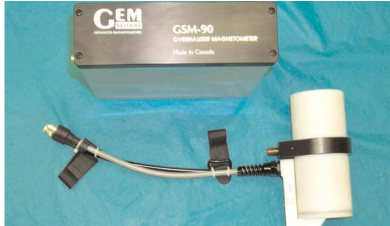
GSM-90 Overhauser Magnetometer console with new sensor for enhanced robustness and signal quality.
