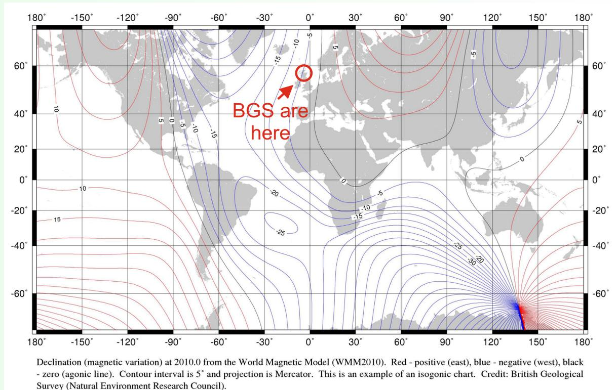
2. Using a map of declination (provided by BGS and NOAA) and the GPS coordinates of the phone location, software computes the required angle of correction for true north.
