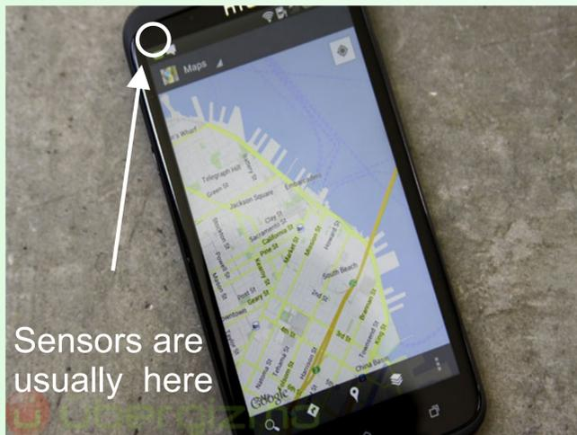
1. Magnetic and gravity field sensors located within your phone measure the direction of **Magnetic North** at the phone's location.
