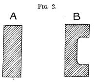
Bars of type A are usually graduated on a vertical face, and the magnet carriage, which possesses a groove sliding on the bar, bears a reference mark—answering to the centre of the magnet—which is brought into coincidence with the scale divisions.
